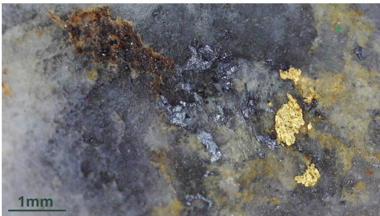
Figure 1: St Arnaud Comstock visible gold, galena and sphalerite (25NED002)
