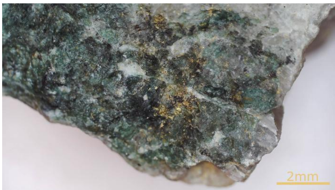
Figure 1: Chip containing visible gold RD046 681.45m (this visible gold section of RD046 is fully assayed, results for rest of hole remain pending).
